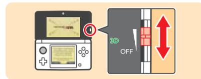
Touch ACTIVATE 3D and the images shown on the upper screen will appear in 3D. Use the 3D depth slider to adjust the 3D effect to a comfortable level, then touch DONE.
