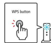
Press and hold the WPS button on the access point until the LED blinks.
